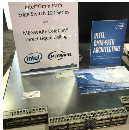
Figure 2: Water cooling on a Omni-Path switch, from MEGWARE..
